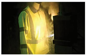
IEC61482-1 and the identical EN 61482-1 are split into two separate parts which cover the methods for testing of fabrics and garments that are designed to protect against the thermal hazards of an Arc Flash.
